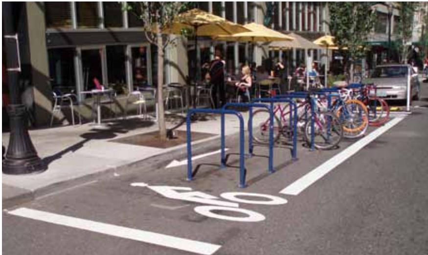
Figure 5.4: Converting parking spaces for bicycle parking is a low-cost, high-visibility approach to increasing bicycle parking supply.
