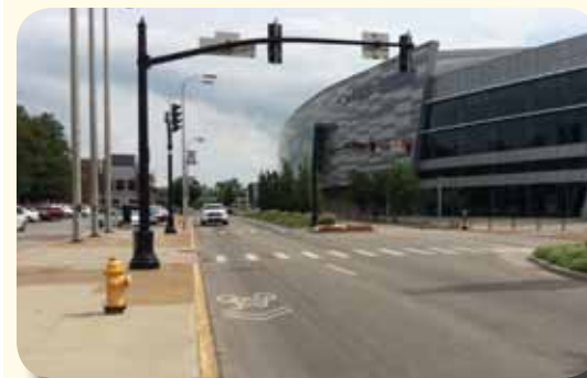
Figure 2.10: These improperly placed shared lane markings along MLK Blvd encourage bicyclists to ride against the curb rather than the middle of the lane, where cyclists can remain visible, predictable, and more safe. (location: MLK Blvd)
